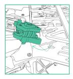
To remove, pinch the cartridge latch to unlock it from the battery and chassis plate, and slide it outwards to disengage. Simultaneously pull the battery and chassis plate apart while pulling the cartridge outward.
