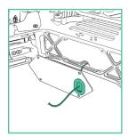
4. Connect the cable to the external voltage sense port on the primary Futaba receiver.
