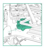
To install, place the cartridges between the top chassis plate and the battery plate. Ensure they are engaged in the track features and are parallel with the chassis and battery plate. Push inwards fully until they click, indicating the cartridges are locked in place. Pull outwards on the cartridge to ensure it is locked in place.
