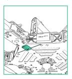
**8.** For Futaba receivers, feed antenna wires into antenna tubes and zip tie to noted mounting location
