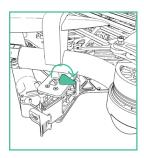
3. Open ALTA 6 booms. ALTA 6 can become unbalanced and tip over while unfolding booms individually, so unfold opposite boom pairs simultaneously to keep balance.
